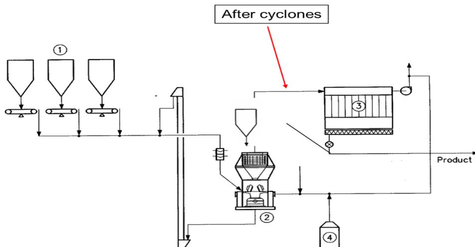
Gas flow measurement with McON Air on outlet of raw mill
