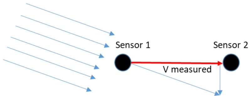
Correlation measurements are vector measurements:  $V$  measured is the distance (Vector) divided by time.
