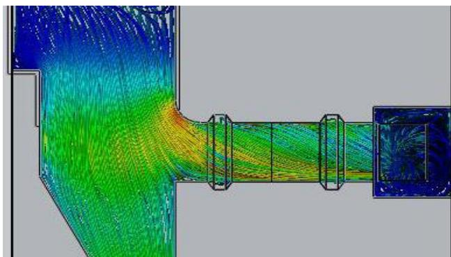
CFD example of swirled flow, which can be measured correctly with correlation measurement systems
